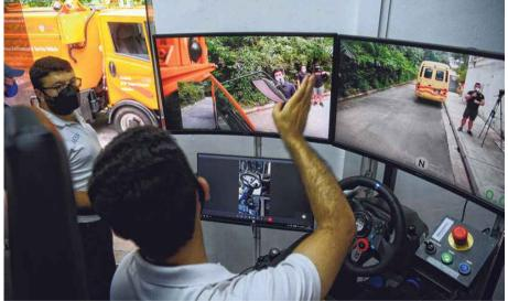
A member of Nanyang Technological University's tele-ops research team demonstrating during a media preview in Sentosa on Monday how a driverless road-sweeping vehicle can, in an emergency, be controlled by an operator at a different location via a tele-operation system. ST PHOTO: MARK CHEONG
